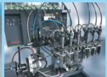
Common Rail Injector Calibration
